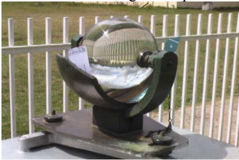
Figure 4.4: Campell sunshine recorder for measuring sunshine duration
