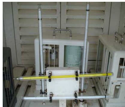
Figure 4.2: Maximum (upper horizontal) and Minimum (lower horizontal) thermometer
