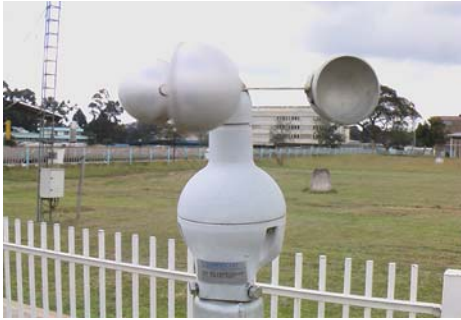
Figure 4.3: Cup- counter anemometer for measuring wind speed
