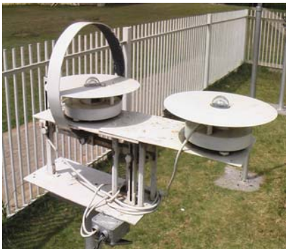
Figure 4.5: Solarimeter for measuring solar radiation
