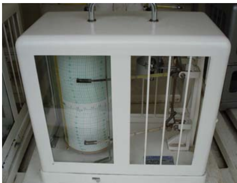
Figure 4.1: Thermo hygrograph for measuring Humidity
