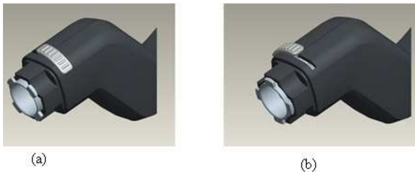
Figure 4.5: Release-switch of antenna module HE300 (a) locked, (b) unlocked
