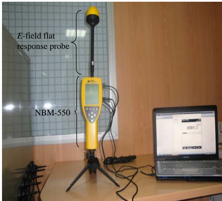
Figure 4.2: Measurement of data from Broadband RF meter – NBM-550
