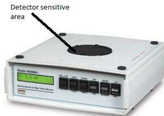
Figure 4-1: The Multimeter used in the current work (The Model 4000M+).
