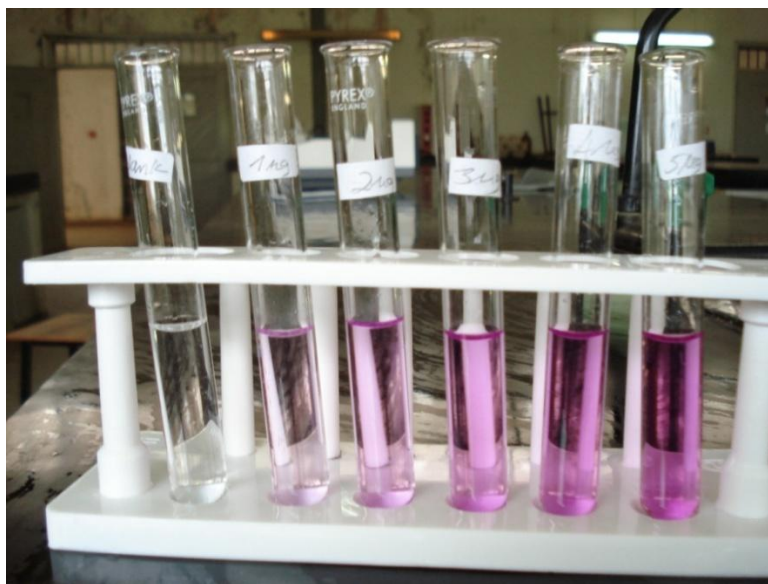
Plate 9: A photograph of test tubes in a test tube rack containing standard nitrite solutions and NO 2 -colouring reagent
