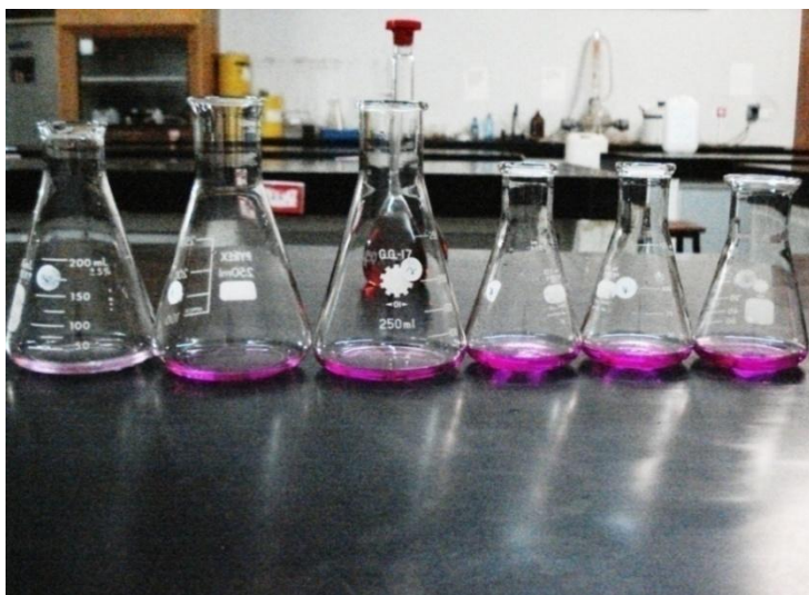
Plate 10: A photograph of conical flasks with a mixture of Sulphite-TCM solutions and \text{SO}_2 -colouring reagent
