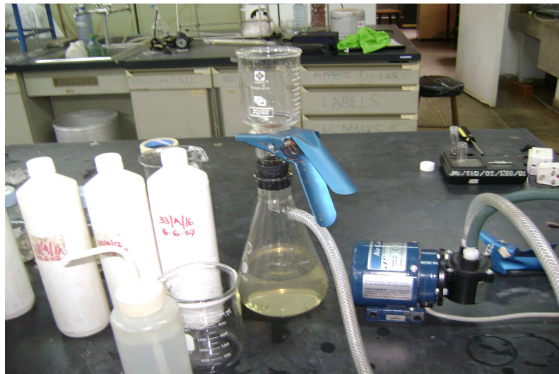
Figure 4. 10. Vacuum filtration apparatus for determining Total Suspended Sediment.
