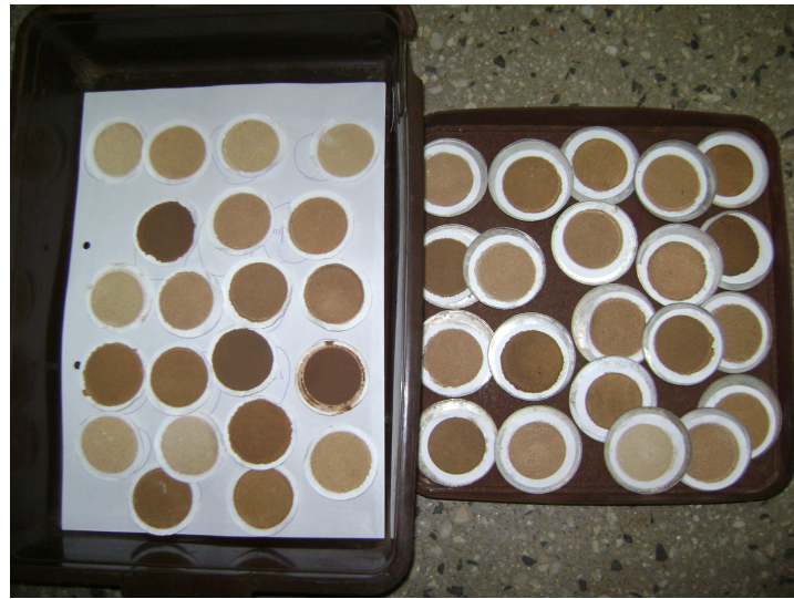
Figure 4. 12. Dried product samples used in X-Ray Fluorescent analysis for trace metals.
