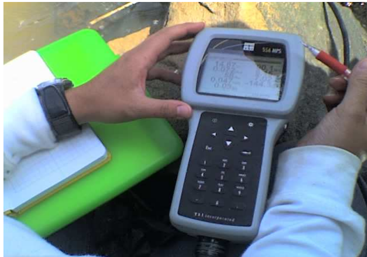
Figure 4. 19. Measuring various parameters using YSI 556 handheld multimeter probe.
