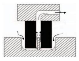
Fig. 5. Suction flushing
