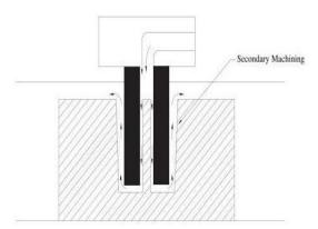
Fig. 3. Effect of secondary discharge machining
