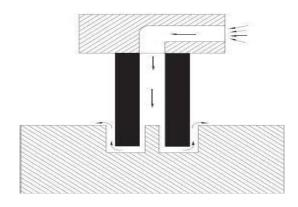
Fig. 1. Pressure flushing through the electrode
