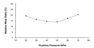
Fig. 7. Effect of flushing pressure on relative wear ratio [11]
