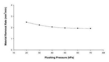
Fig. 6. Effect of flushing pressure on material removal rate [11]
