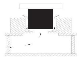
Fig. 2. Pressure flushing through the workpiece
