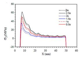
Fig. 5. Stresses distribution simulation results along the grooved crack tip (y=0, z=0.548 mm). [15]
