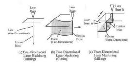
Fig. 1. Schematic showing one, two and three dimensional laser machining [6]
