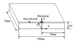
Fig. 4. Half of the glass substrate and the coordinate system [15]
