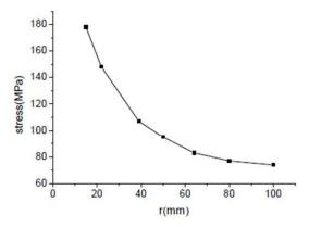
Fig. 7. Plot of maximum stress for different preheating laser diameters. [18]
