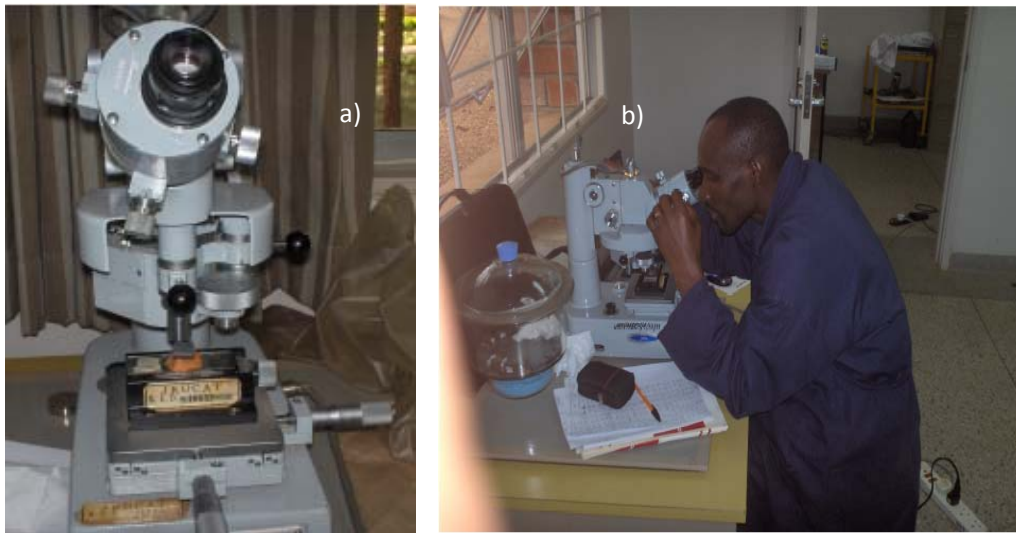
Figure 3.17: Microvickers hardness tester used in determination of hardness, a) specimen under load, b) reading of imprint indentation
