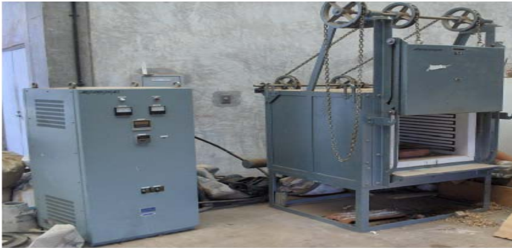
Figure 3.12: Electrical Muffle Furnace used for heat treatment (1200 °C Maximum capacity) at JKUAT, Structural and Materials Engineering lab
