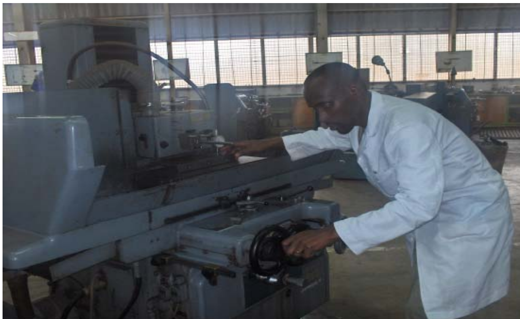
Figure 3.7: Surface grinding of metallographic specimen
