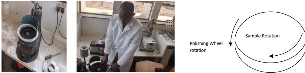
Figure 3.9: Polishing operation with diamond paste on a rotating wheel polishing machine
