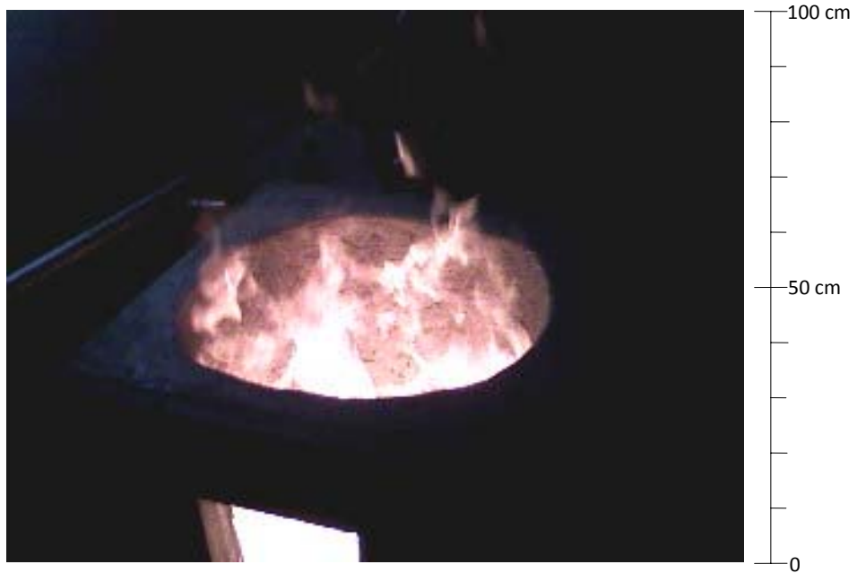
Figure 4.5: Flame length in the final combustion chamber
