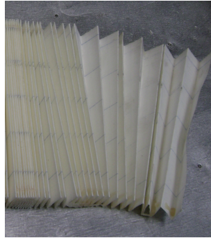
Figure 5.2: A defective panel filter element
