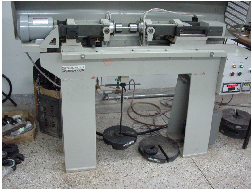
Figure 3.4: A photograph of Ono's high temperature rotary bending machine used for fatigue testing.
