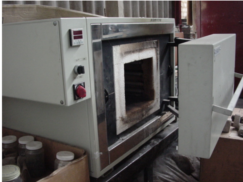
Figure 3.3: A photograph of the air circulated electric resistance furnace used for heat treatment.
