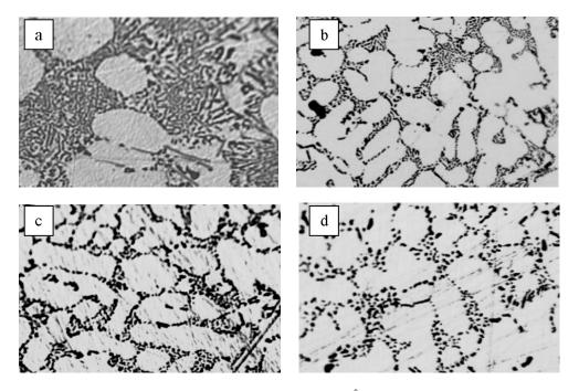
Figure 3. Microstructures for the section with the cooling rate of  $2.11^{\circ}$ C/s (a) in the as cast state (b) after solution treatment 30 minutes at  $540^{\circ}$ C (c) solution treatment of 1 hour and (d) solution treatment of 6 hours.
