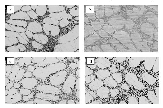
Figure 5. Microstructures for the section with the cooling rate of 0.98°C/s (a) in the as cast state (b) after solution treatment 30 minutes at 540°C (c) solution treatment of 1 hour and (d) solution treatment of 6 hours.
