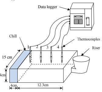
Figure 1. The data logger, casting and thermocouple assembly
