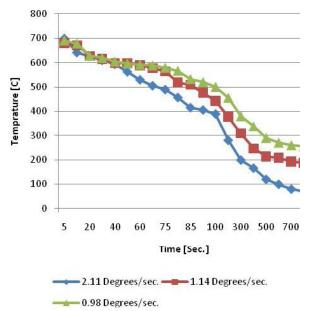
Figure 2. The cooling curves of the different sections of the casting.
