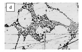
Figure 4 Micrographs (a) in the as cast state (b) after 30 minutes solution treatment (c) after 3 hours and (d) after 6 hours solution treatment for the section with a cooling rate of 1.14°C/s.
