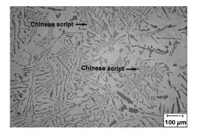
Fig. 6. Microstructure of the Mn-modified alloy containing 1.8 per cent Fe.
