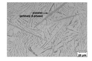
Fig. 4. Microstructure of unmodified alloy containing 1.4 per cent Fe.
