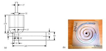
Fig. 2. The experimental setup for fluidity test.
