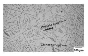
Fig. 5. Microstructure of the Mn-modified alloy containing 1.4 per cent Fe.
