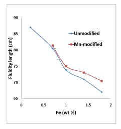
Fig. 3. The effect of Fe on the fluidity of un-modified and Mn-modified alloys.
