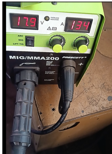
Figure 3.2: MMA/MIG/TIG 200 Prescott Welder
