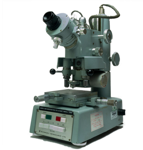
Figure 3.9: Shimadzu Micro Hardness Tester
