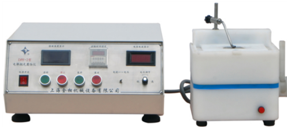
Figure 3.8: MEP-2 Metallographic Polishing Machine
