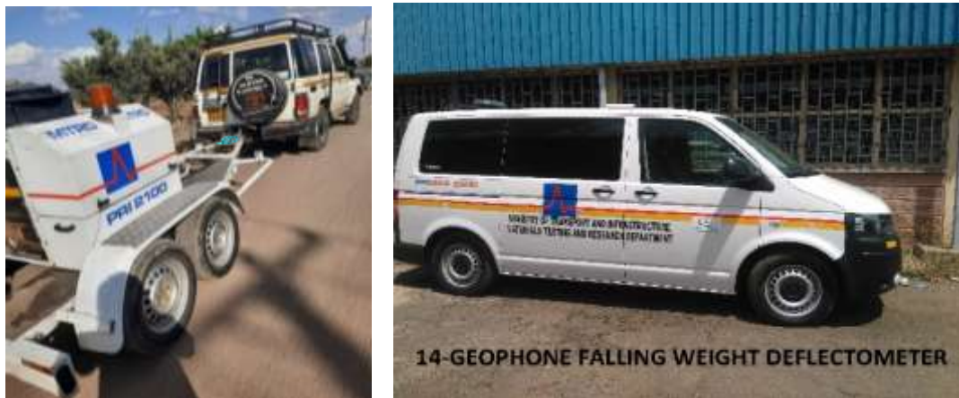
Figure 3.2: 9- and 14-geophone FWD (Primax, Germany)
