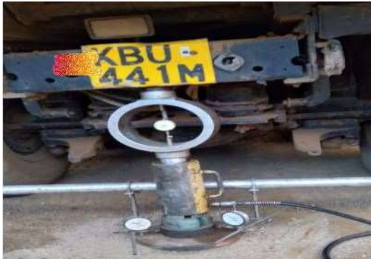
Figure 3.3: Plate Bearing Test apparatus
