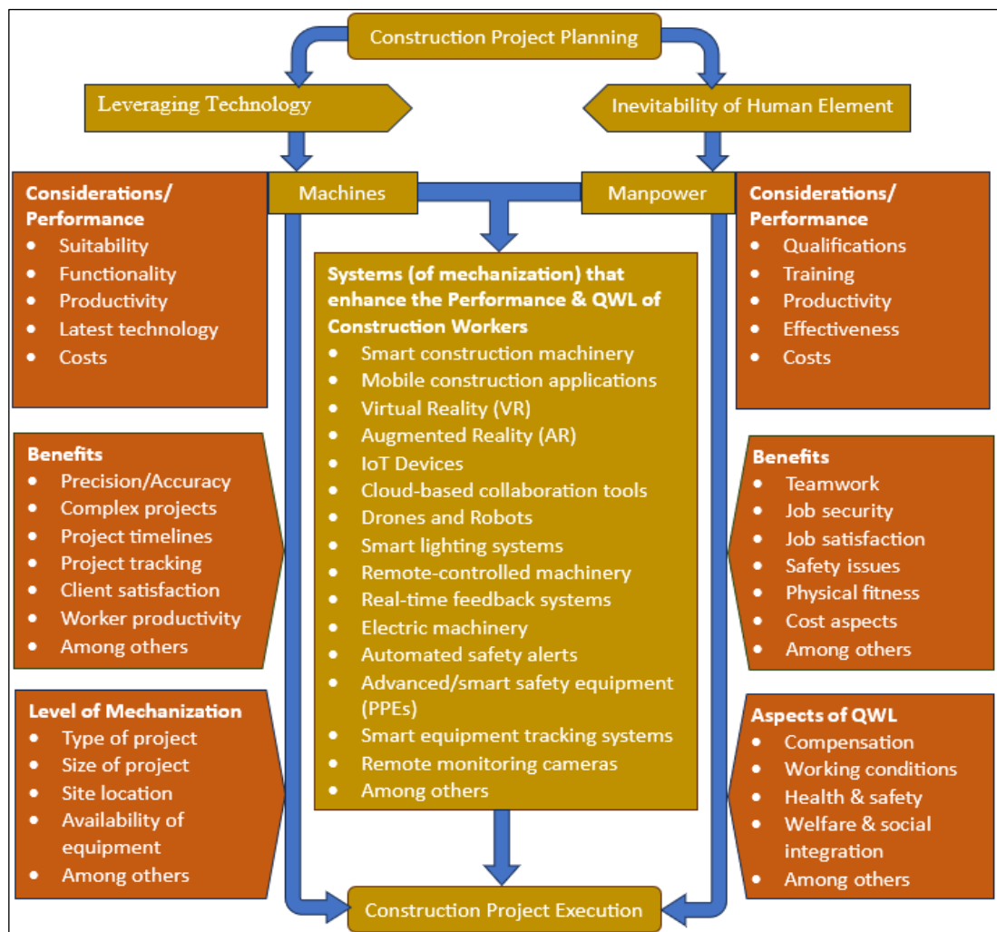
Figure 4.9: A Framework for Optimizing the Level of Mechanization and Manpower in Construction Projects in Kenya
