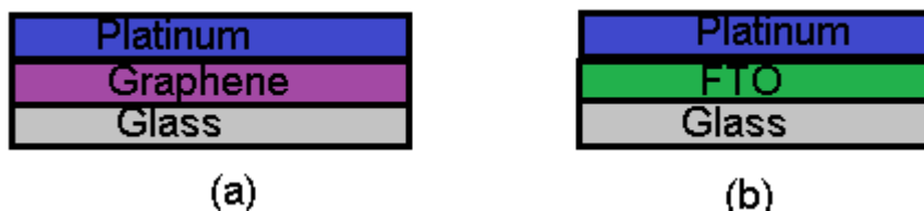
Figure 3.3: Schematic Diagrams of the CE Modules Prepared, Showing (a) Glass/Gr/Pt (b) Glass/FTO/Pt
