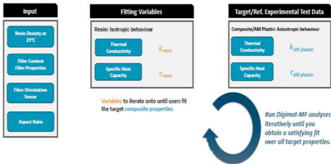
Figure 3.7: Calibration of the Thermal Conductivity and Specific Heat Capacity of the Resin on the Thermal Material Card
