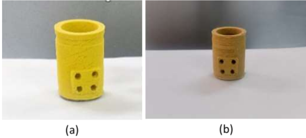
Figure B. 3: Printed adapter of the breath analyzer (a) 100 wt.% rHDPE (b) bioplastic
