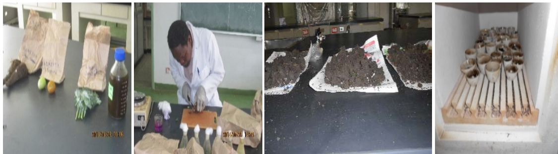
Figure 3.2: Initial preparation steps for the delivered crop, water and soil samples preparation steps including ashing in a muffle furnace prior to acid digestion.
