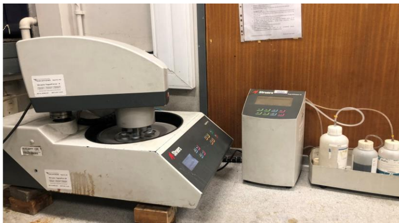
Figure 3.6: Grinding and Polishing Machine at CSIR
