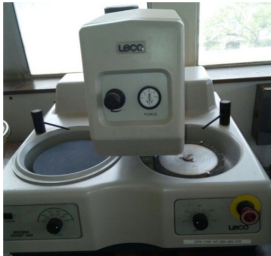
Figure 3.12: Leco machine used for automatic grinding and polishing
