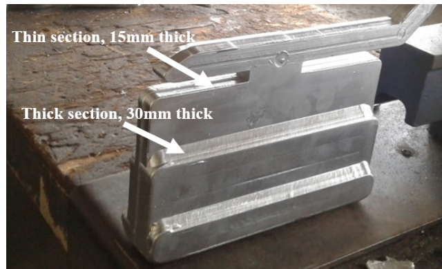
Figure 3.3: Bar casting after melt solidification in permanent mold
