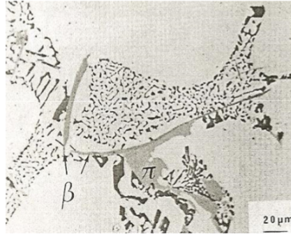
Figure 2.5: \beta - \text{Al}_5\text{FeSi} and \pi - \text{Al}_8\text{Mg}_3\text{FeSi}_6 Fe-phases in as-cast Al-7Si-0.3Mg-0.52Fe alloy (Gustafsson et al., 1986)
