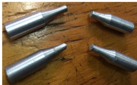
Figure 3.6: Failed specimens before 10^7 cycles during the experiment
