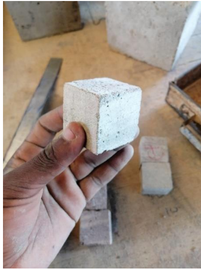
Figure 3.5: Cement Block Cured for the Determination of Strength Activity Index of Calcined Clay
