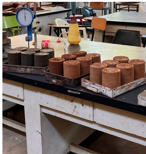
Figure 3.8: Stabilized Blocks Prepared for Compressive Strength Test
