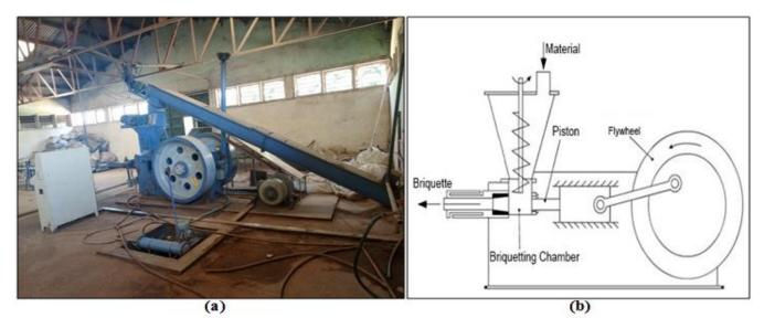
Figure 2: (a) Piston-type briquetting machine and (b) Piston-type machine diagram
