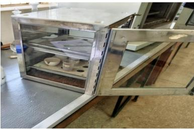
Figure 5: Desiccator containing desiccant
