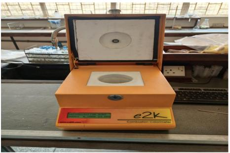
Figure 6: e2K Combustion Calorimeter
