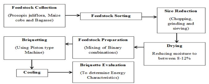
Figure 1: Briquetting Process Flowchart
