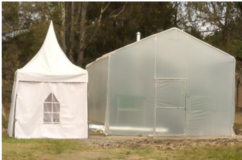
Figure 1: A photograph of the greenhouse solar dryer used in the study.
