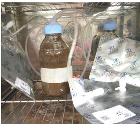
Fig. 1 CSTRs laboratory set-up in the incubator
