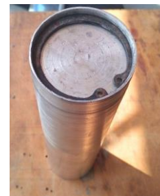
Fig. 14. Bulkhead fitted into casing
