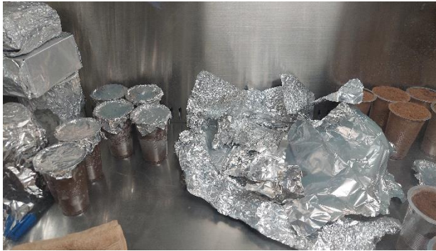
Plate 4.1: Packing sterilized sand into sterilized containers under sterilized cabinet equipped with laminar airflow to prevent cross-contamination
