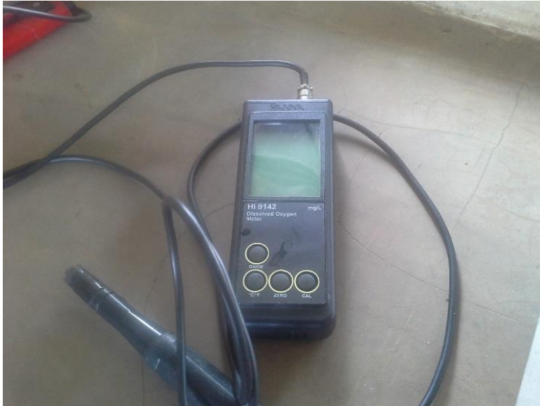
Plate 3.3: Hanna DO meter used to record dissolved oxygen readings
