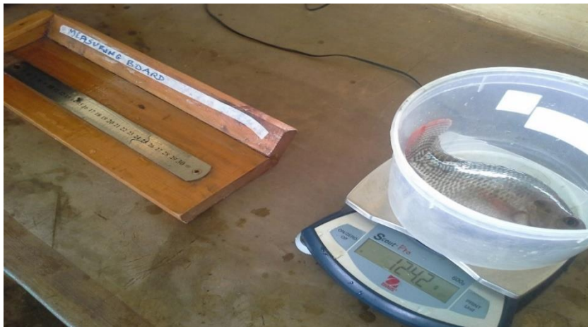
Plate 3.2: Measuring board (on the left) and electronic weighing scale (on the right) with a fish specimen on it
