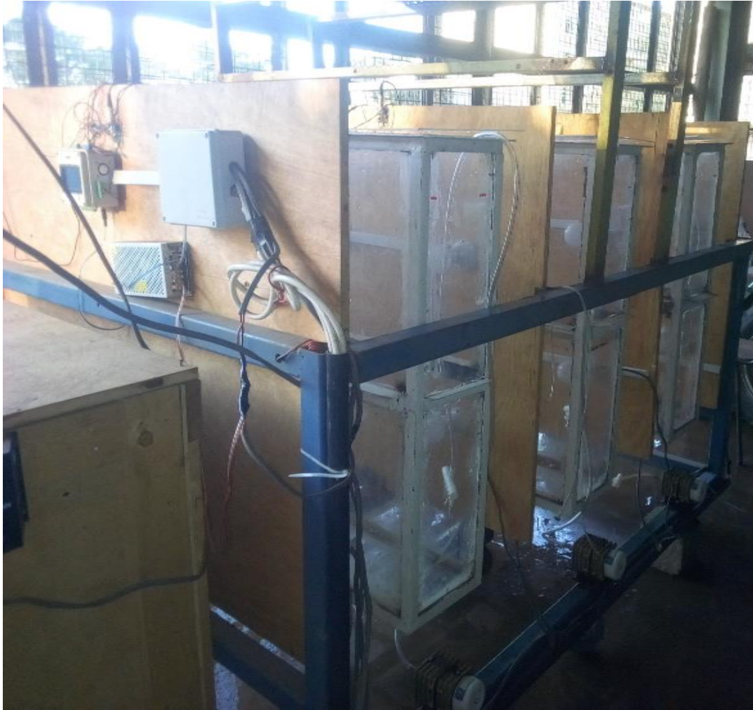
Figure 3.2: Flat Plate Perspex Photobioreactor Used in the Study
