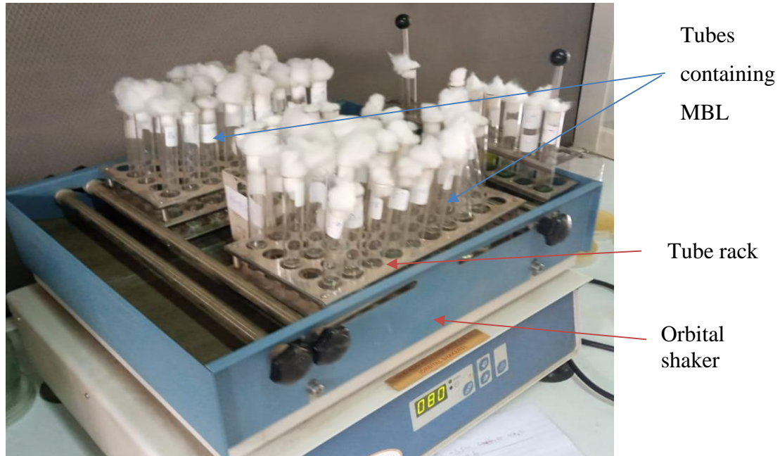
Figure 3.10: Experimental Setup for Isolation by Serial Dilution Method in MBL
