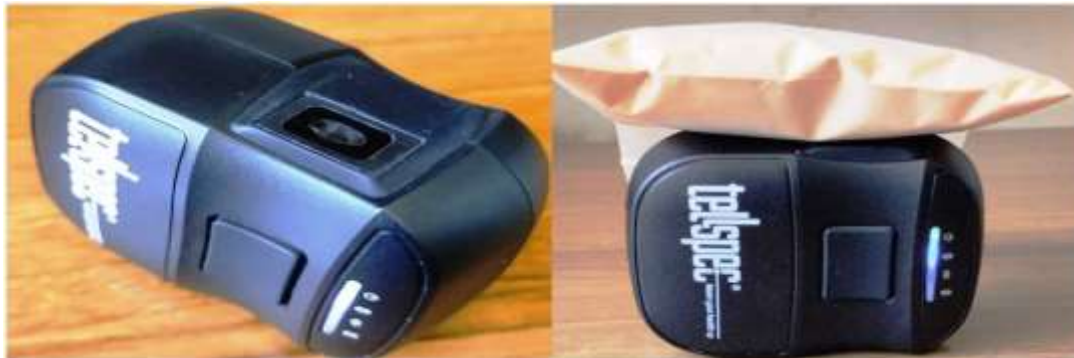
Figure 2.2: Portable/handheld NIR spectrometer (Model: NIR-S-G1, Telspec, Toronto, Canada).
