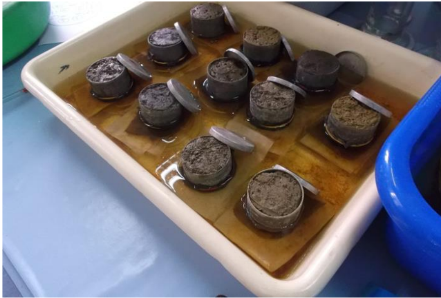
Plate 3.1: Saturation of the undisturbed Soil Samples
