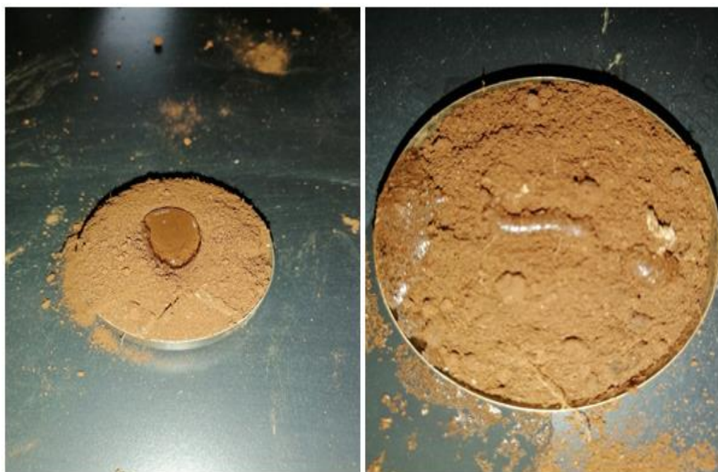
Plate 3.2: WDPT-Test Showing behavior of Water Droplet on Repellent Soil Sample
