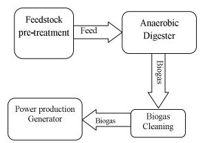
Figure 1 Biogas Production Sequence
