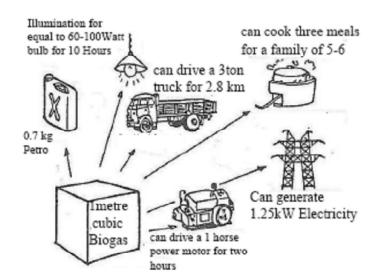
Figure 2 Energy Equivalence of One Cubic Meter of Biogas
