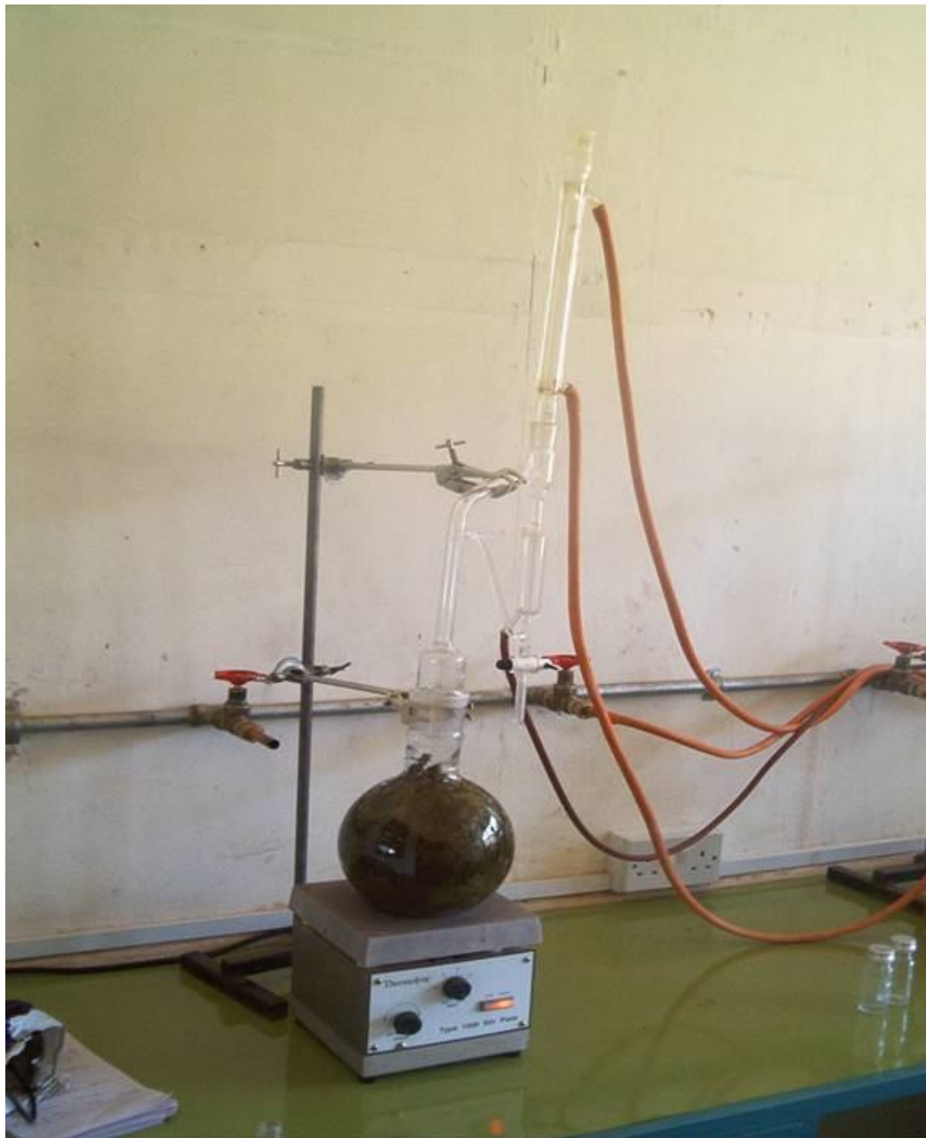
Figure 7.0: Hydro distillations of essential oils from Ocimum gratissimum in a Clevenger- type apparatus
