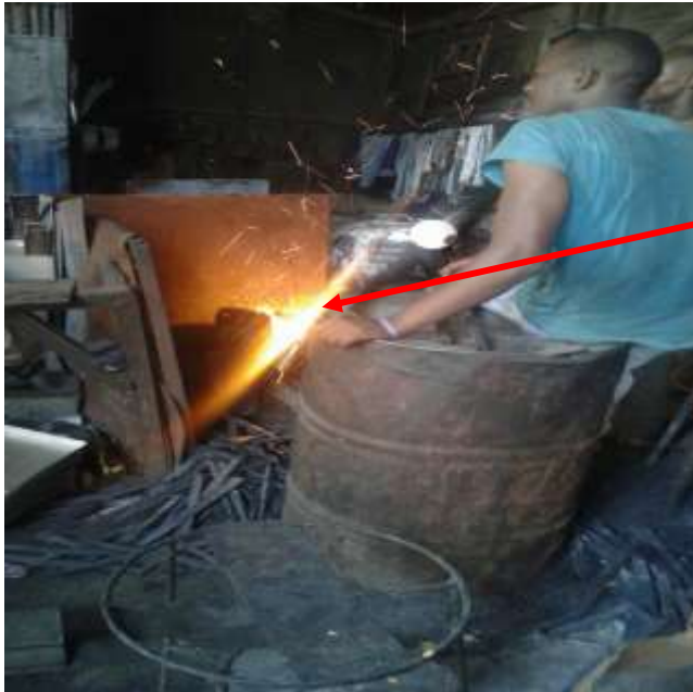
Plate 4.1: Open Heating of Scrap Metal to Make it Malleable
