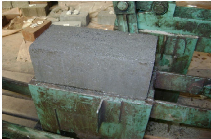
Plate 3.5 Laterized quarry dust block being removed from the machine
