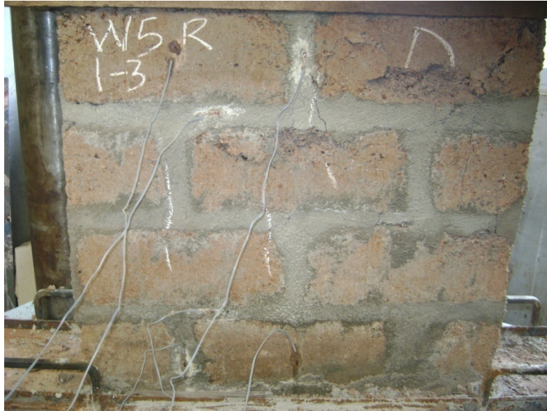
Plate 8.3: Cracking pattern for reinforced alternative block wall utilizing 1:3 jointing mortar
