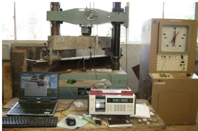
Plate 3.4 Experimental set-up of concrete beam ready for testing
