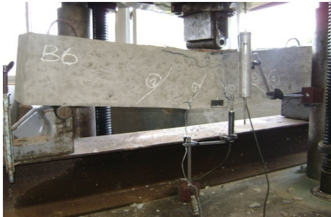
(b) Final cracks pattern at ultimate load
