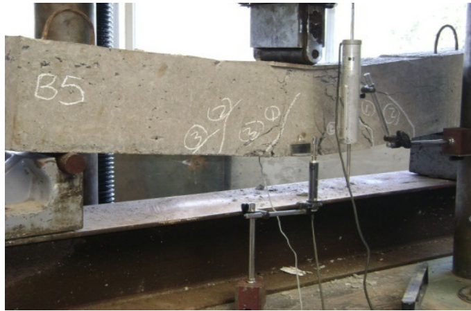
(b) Final cracks pattern at ultimate load
