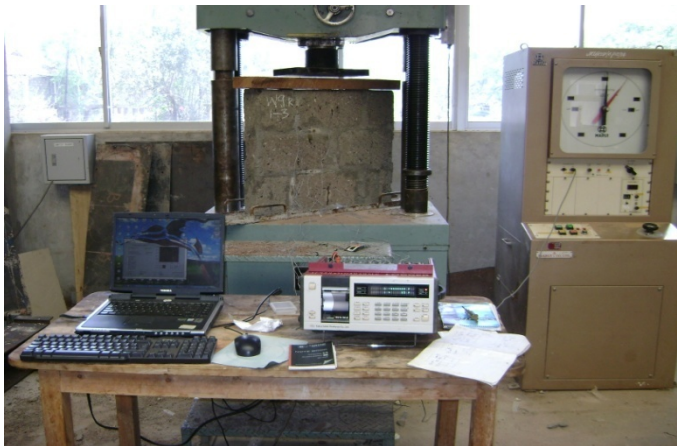
(b) Photo of experimental set-up for wall panels
