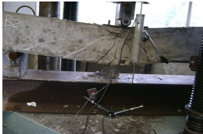
(b) Final cracks pattern at ultimate load
