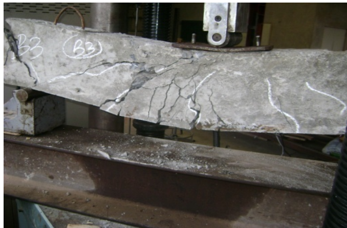
(b) Final cracks pattern at ultimate load
