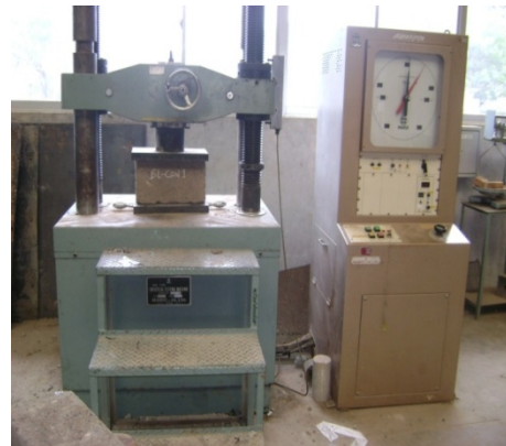
Plate 3.3 Experimental set up for testing blocks on a UTM.
