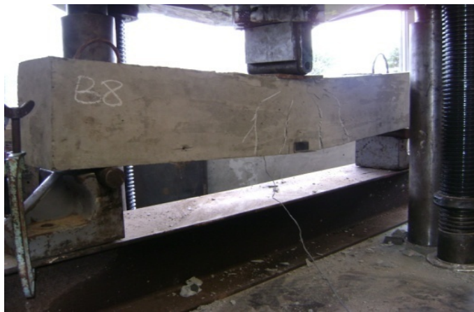
(b) Final cracks pattern at ultimate load
