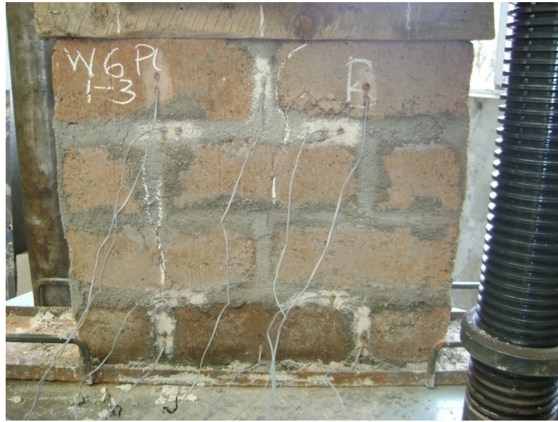
Plate 8.4: Cracking pattern for plain alternative block wall utilizing 1:3 jointing mortar
