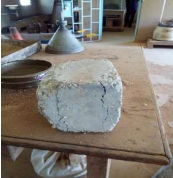
Plate 3.8: concrete cubes after failure on compression loading
