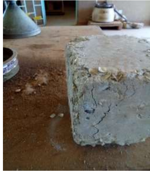
Plate 3.8: concrete cubes after failure on compression loading
