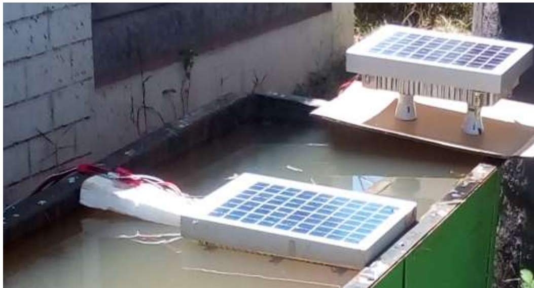
Figure 3.6: PV Module Temperature and Voltage Measurement
