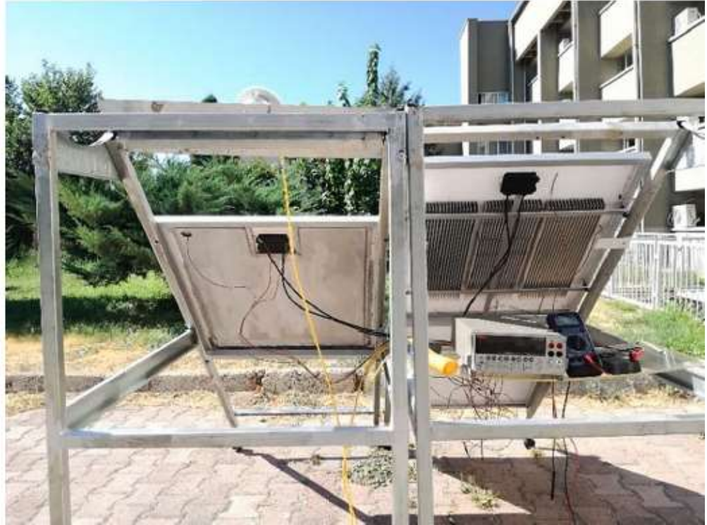
Figure 2.4: Back view of the PV setup (left) PV + PCM (top right) PV + Fin (bottom right) Reference PV (Bayrak et al., 2020)
