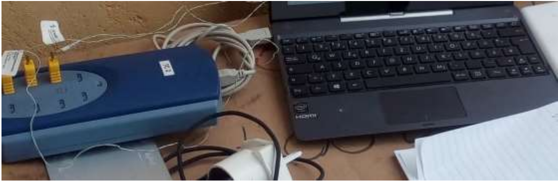
Figure 3.16. PV Module Temperature and Voltage Measurements
