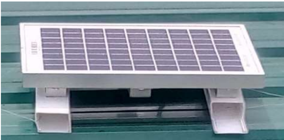
Figure 3.13: PV Module Temperature Measurement
