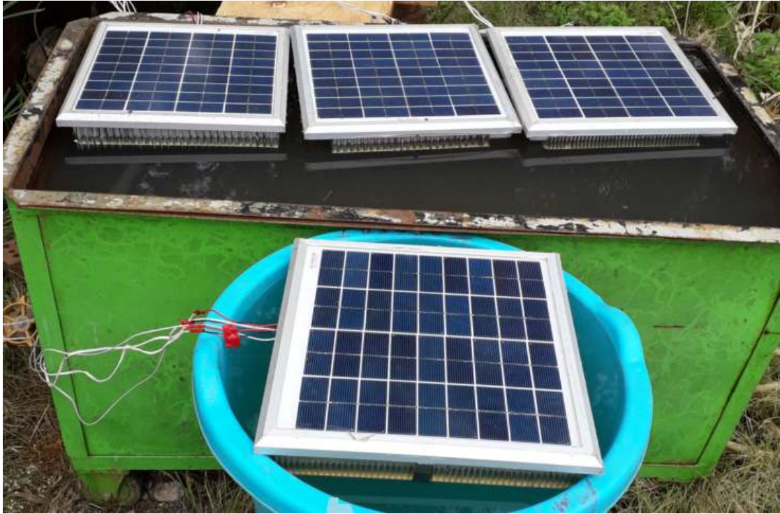
Figure 3.31: Water cooled PV-TEGs setups for the three TIMs and the reference case
