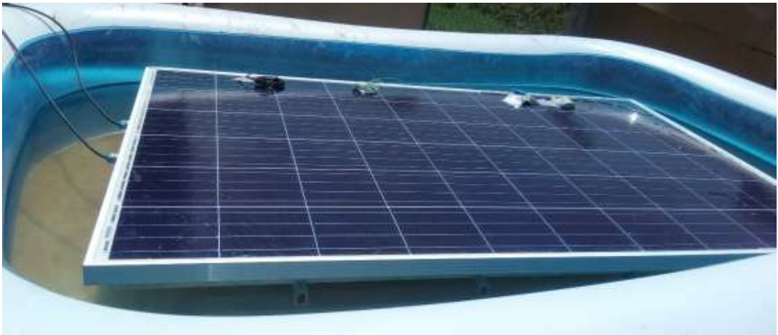
Figure 3.15.: PV Module Temperature and Voltage Measurements
