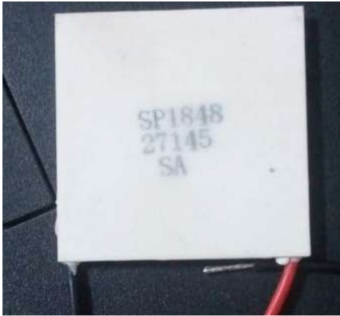
Figure B 8. Thermoelectric generator Module
