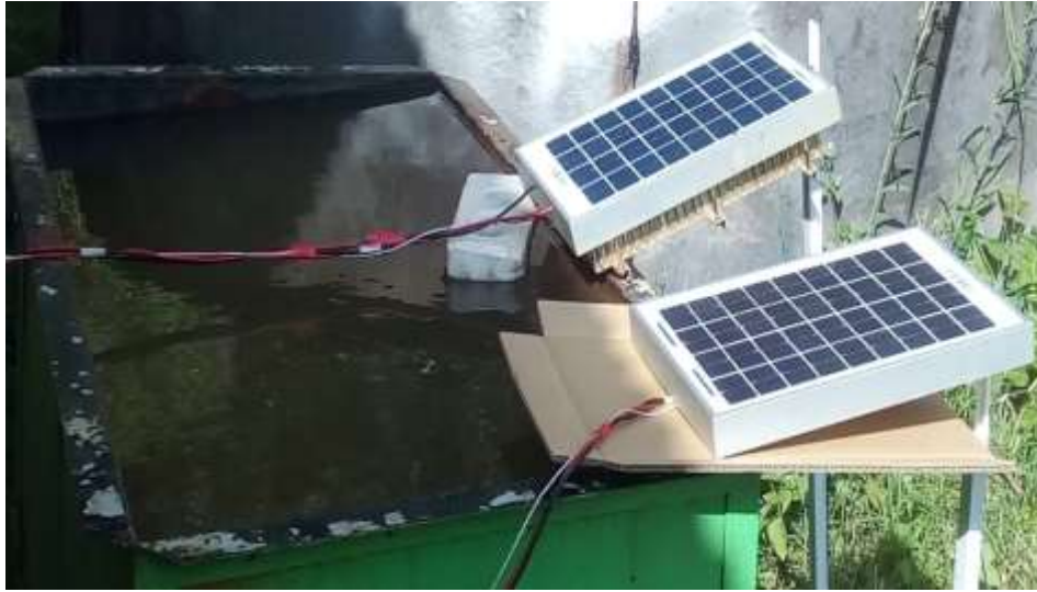
Figure 3.4: PV Module Temperature Measurement under Air Cooling
