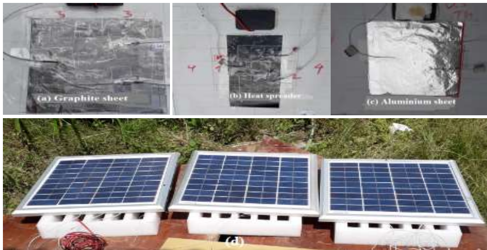
Figure 3.29: Systematic temperature distribution measurements using various TIMs; (a) Graphite (b) Heat spreader (c) Aluminum foil (d) Complete setup of the three sets.
