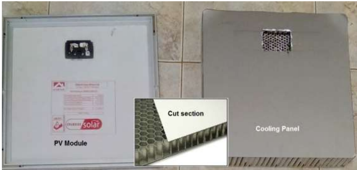
Figure B 9. Alucore cooling panel (RHS) ready for mounting
