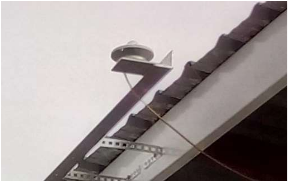
Figure 3.11: CMP-3 Pyranometer in Nyalenda Kisumu
