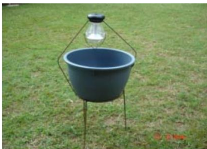
Figure 2.1: The termite harvester showing light source, collector basin and stand. Source: Ayieko et al. (2011).
