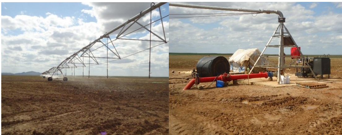
Plate 2.2: Center pivot irrigation system at Galana Kulalu Irrigation Scheme (National Irrigation Board), Kenya (source: author, 2015)
