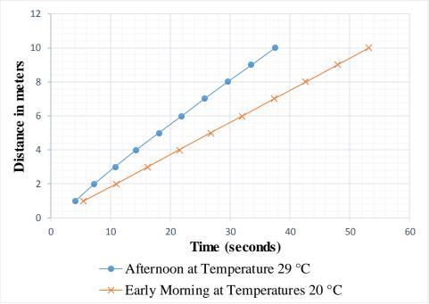
Fig. 4: A plot of distance (meters) against time (seconds) showing the response of the system when using Rose Fragrant Perfume measured at 20°C and at 29°C.
