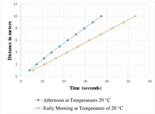
Figure 5: A plot of distance (meters) against time (seconds) showing the response of the system when using Lavender Fragrant Perfume measured at 20°C and at 29°C.
