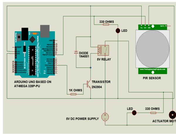
*Fig. 1: Circuit diagram showing the connection of the system components making up an entry alert system for the deaf-blind.*
