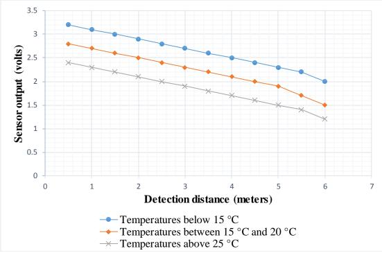
*Fig. 3: A graph of sensor output against detection distance showing the inverse relationship between temperature and PIR sensor sensitivity.*
