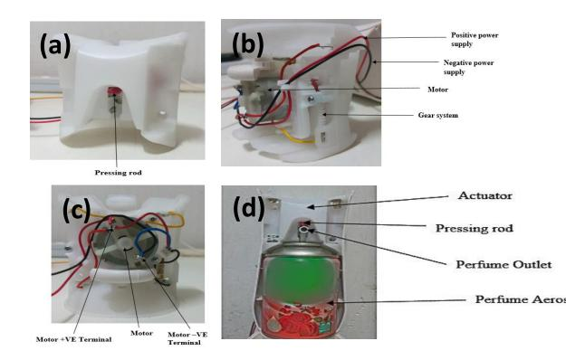
Fig. 2: (a) Front view, (b) Side view (c) Back view and (d) the actuator system and aerosol containing rose fragrant perfume fitted in the actuator element.
