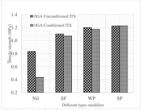
Figure 3: Tensile strength of modified open graded asphalt concrete
