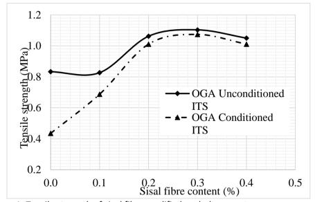
Figure 1: Tensile strength of sisal fibre modified asphalt concrete
