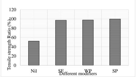
Figure 4: Tensile strength ratios for asphalt concrete with different additives
