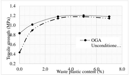
Figure 2: Tensile strength of waste plastic modified open graded asphalt concrete
