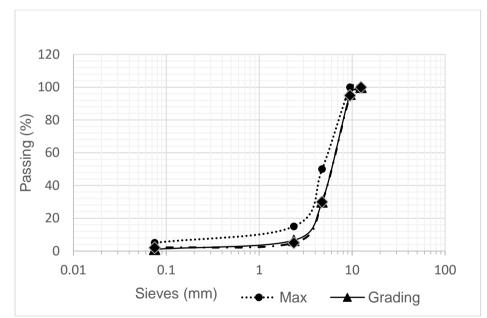
Figure 1: Grading curve for 6/12 mm aggregate for OGA mix.
