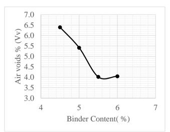
Figure 2(c): Bitumen content vs % Air voids
