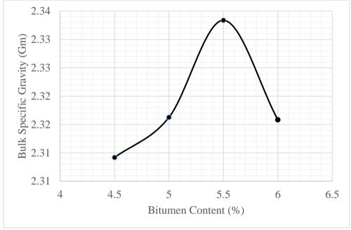
Figure 2(a): Bitumen content vs density of mix.
