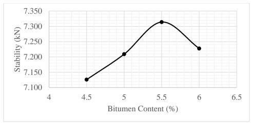
Figure 2(b): Bitumen content vs stability.
