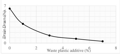
Figure 3(b): Variation of draindown with different percentages of waste plastics.
