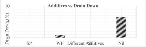
Figure 4: Draindown results for different additives
