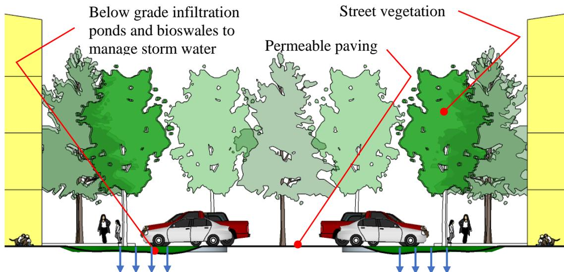
**Figure 4.62: Below Grade Bioswales, Retention and Infiltration Ponds in Medium Density Neighbourhoods**
