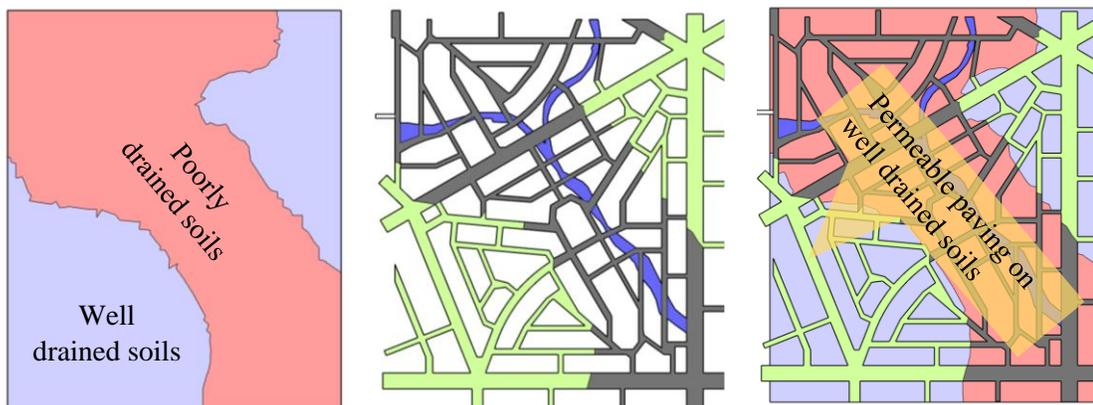
**Figure 4.61: Distribution of Permeable Paving on Well Drained Soils**
