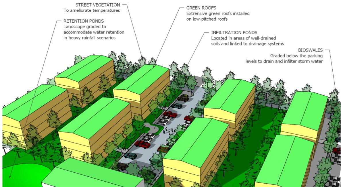
**Figure 4.63: Climate Adaptation through Bioswales, Green Roofs, Retention, and Infiltration Ponds at the Medium Density Residential Neighbourhoods**
