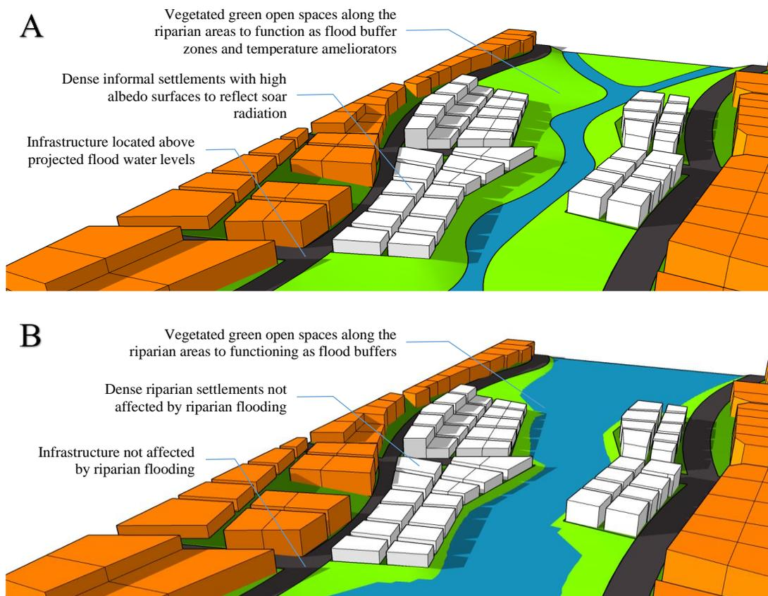
**Figure 4.65: Flood and Temperature Amelioration in Dense Informal and Riparian Settlements**
