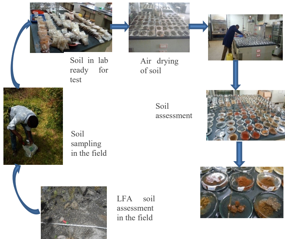
Plate 5.1: Steps followed for soil surface and stability assessment from the field to laboratory.
