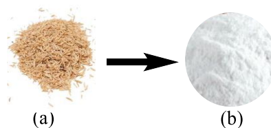
Figure 4.1: Conversion of rice husks (a) to cellulose (b)
