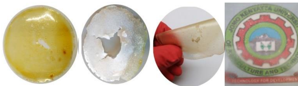
Plate 4.11: Raw CMCS (A), TOCNF-DAC (B), and TOCNF-CMCS-AgNPs (C), TOCNF-DAC-CS films
