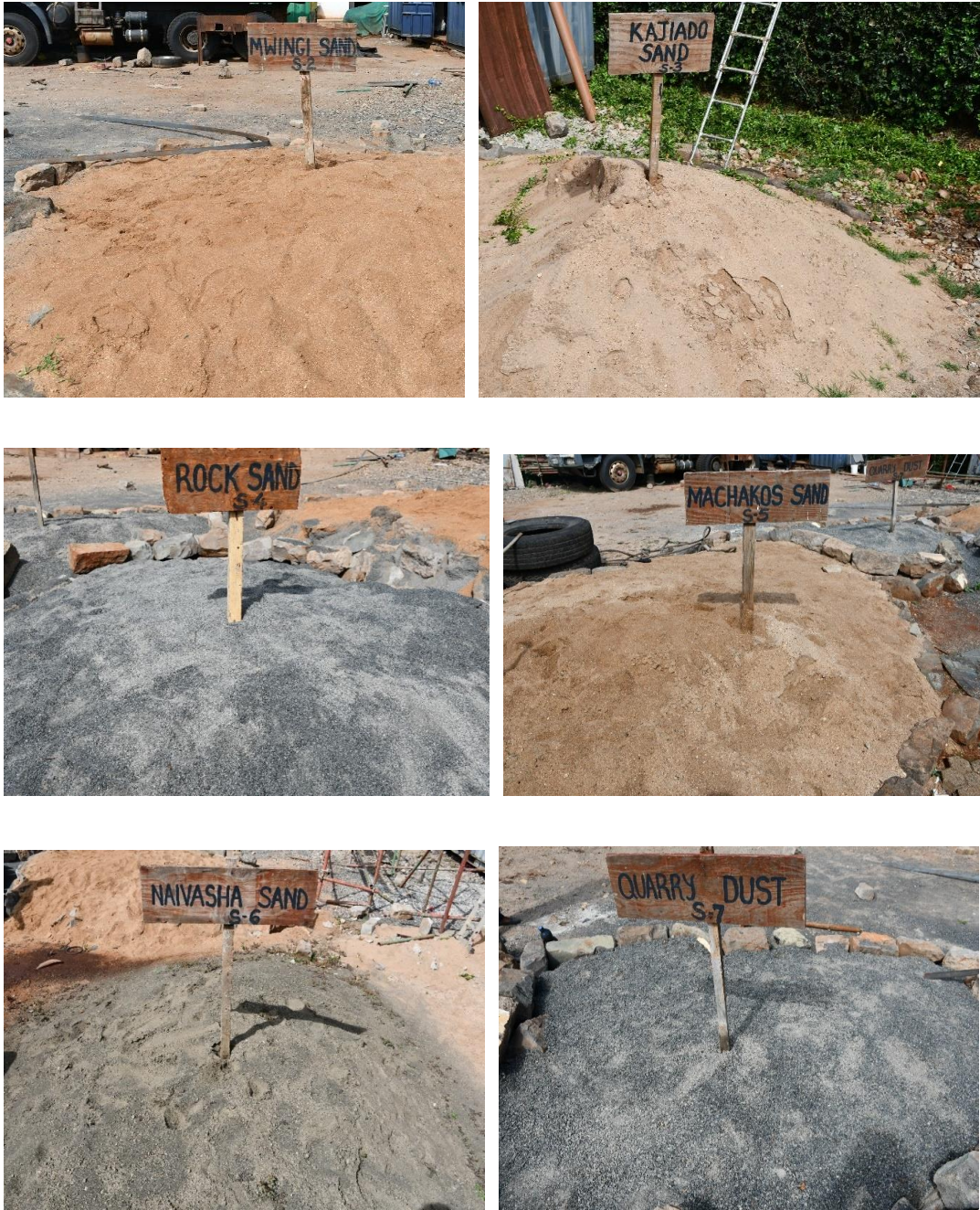
Figure 3.4: Storage of fine aggregates
