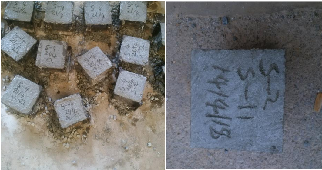
Figure 3.7: Concrete placement and marking
