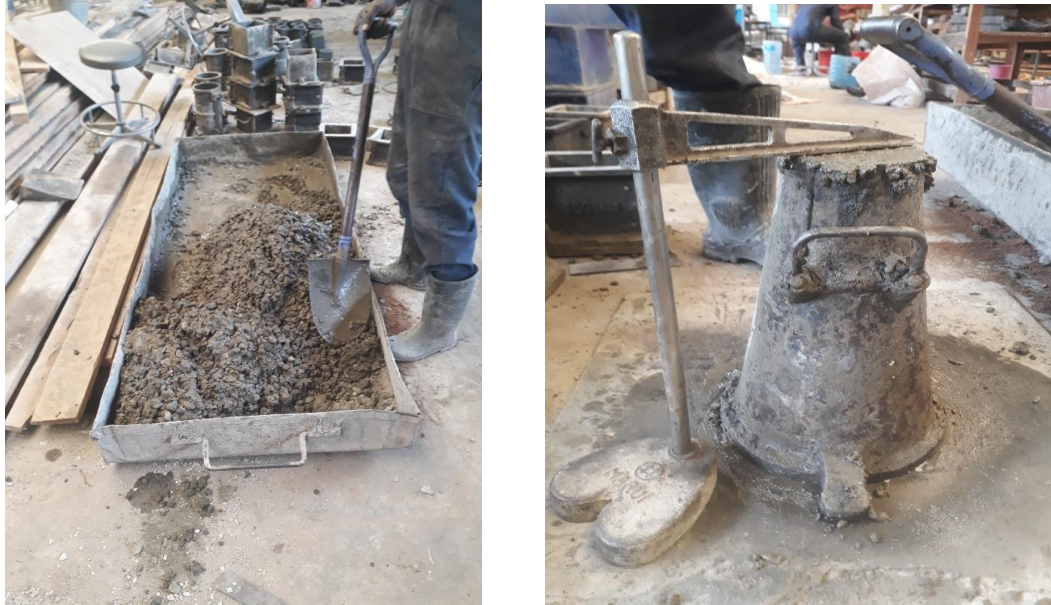
Figure 3.6: Concrete mixing and slump testing
