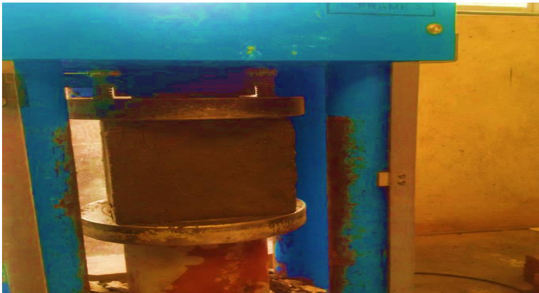
Figure 3.9: Compressive strength testing in the laboratory
