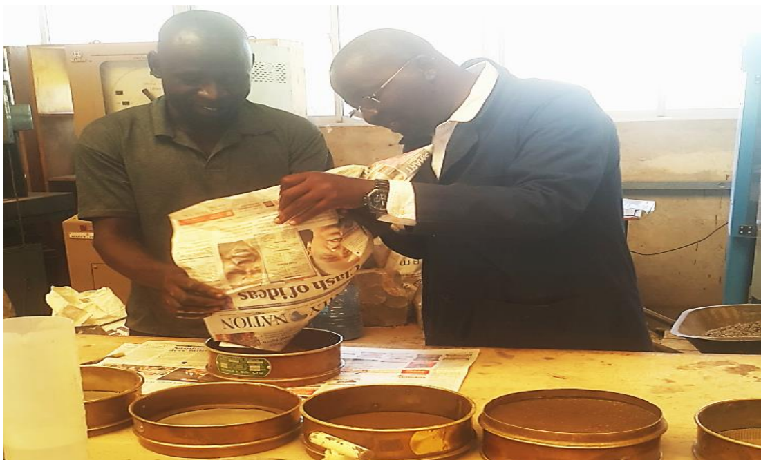
Figure 3.5: Testing of fine aggregates
