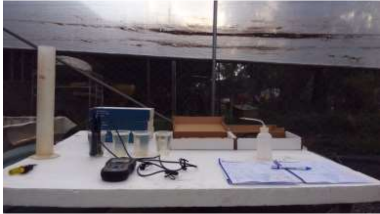
Plate F2: RAS water samples, the multimeter and two probes connected to it during data collection
