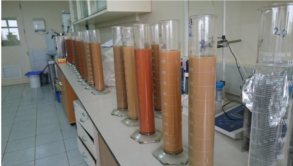
Figure 3.8: Soil texture analysis using the hydrometer method at Mazingira centre lab, ILRI for soils collected at Kirogo Rice Research farm
