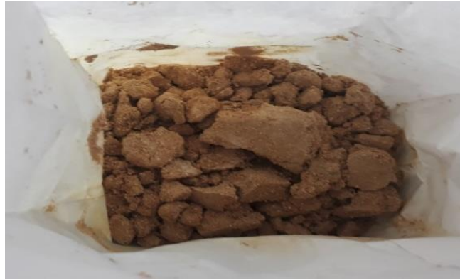
Figure 4.9: Caked sample of ASCF packaged in kraft paper, stored at 35°C and 75%RH
