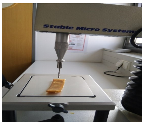
Figure 3.8: Puncture test using a texture analyser (model TA-XT2)
