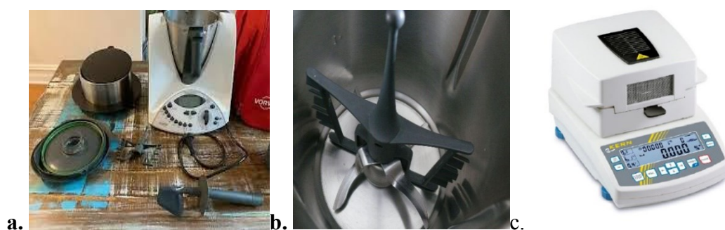
Figure 3.1: (a) Thermomix, (b) mixing whisk installed in Thermomix, (c) Infrared moisture analyzer
